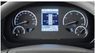
Tyre Pressure Monitoring (TPM) displays the current pressure in the individual tyres and warns of deviations from the optimum pressure. This reduces tyre wear, has a positive effect on fuel consumption and prevents dangerous tyre damage.
