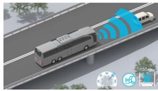
The Adaptive Cruise Control feature (ACC) relieves the driver by maintaining a constant distance – defined by the driver – from the vehicle ahead, based on continuous measurements. This not only increases safety on country roads and motorways, but also convenience.
